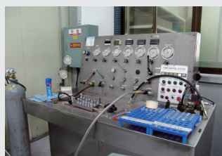
Valve Test Stnad 350kg/cm 2 , 80Lpm
